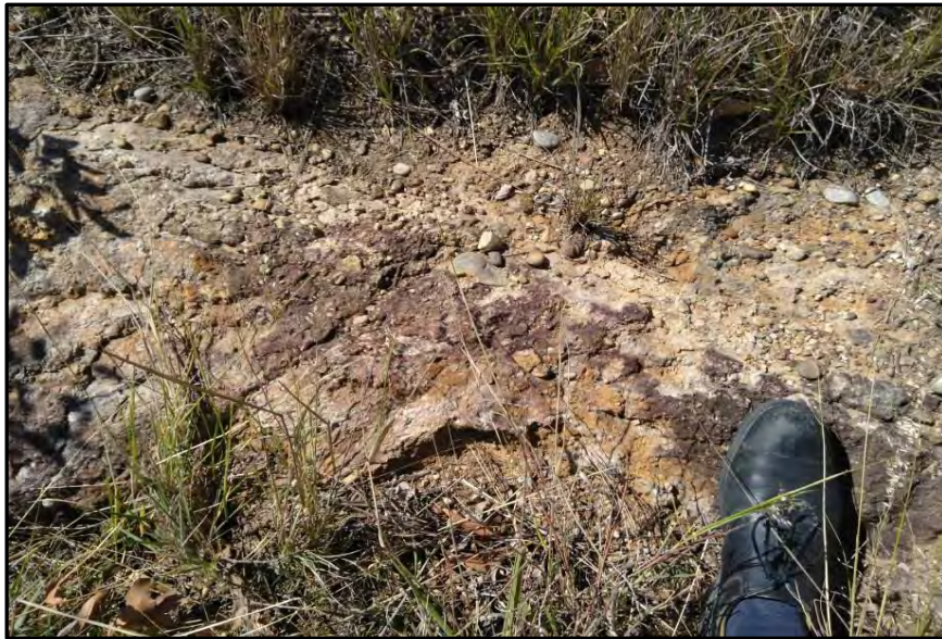
Photo 25: High strength volcanic rock exposed in cutting
