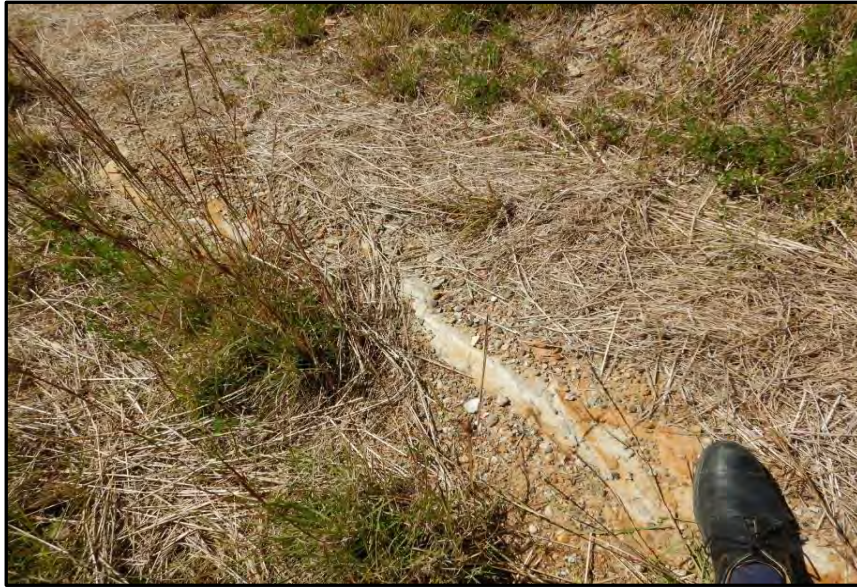
Photo 15: Medium strength sandstone exposed in cutting
